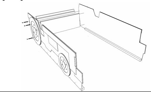
Step 3: Fasten shelf [E] to shelf front section [C] and shelf rear section [D] using screws [H].
