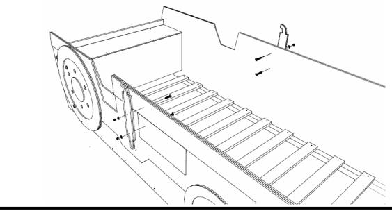
Step 6: Tighten all hardware. Make sure all assembled parts are tight and secure.
