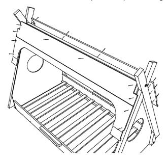
**Step 5:** Fasten bottom panel 1 [I] and bottom panel 2 [J] to frame using short screws [C], (20) per side through pre-drilled holes. Note that each top panel is matched to a bottom panel: both will be marked on the inside either '1' or '2'. These should be placed on the same side.
