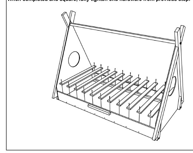
**Step 4:** Fasten top panels [H] to frame using short screws [C], (10) per side through pre-drilled holes. Note that each top panel is matched to a bottom panel: both will be marked on the inside either '1' or '2'. These should be placed on the same side.
