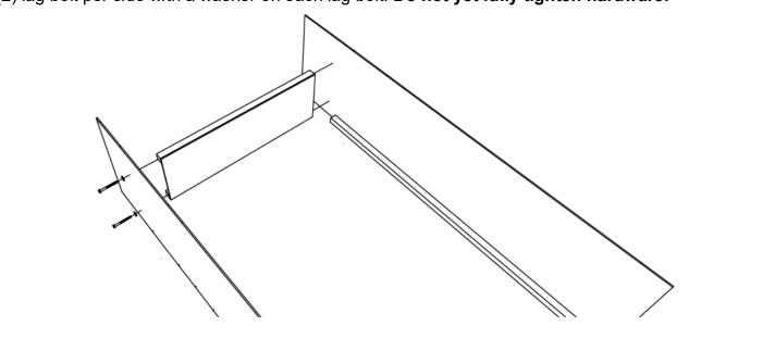
**Step 3:** Fasten mattress support bars [B] to support rail of side assemblies [A] using screws [C]. Use (1) screw at each end of support bar. Support bar end shall be perpendicular with side of bed. There may be a slight gap between end of support bar and side of bed. Start at rear of bed and work towards front. Leave approximately 4.5" gaps between each support bar (approximately 7" center-to-center).
