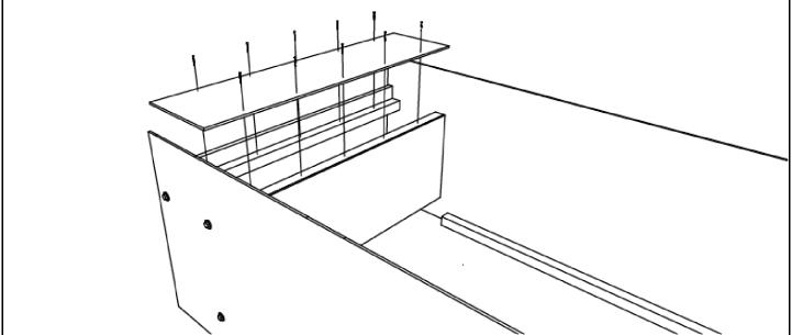
**Step 3:** Fasten mattress support bars [B] to support rail of side assemblies [A] using screws [C]. Use (1) screw at each end of support bar. Make sure support bar end is tight and perpendicular with side of bed. Start at rear of bed and work towards front. Leave 4.5" gaps between each support bar (approximately 7" center-to-center).
