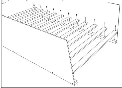
**Step 3 - B:** Fasten auxiliary side assemblies [A3] to side assemblies [A] and attached parts using screws [M]. Side assemblies pictured are for reference only; individual assembly types will vary with bed model. For exact fit and style, refer to picture on cover of manual.
