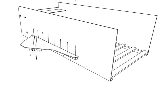
**Step 3 - J:** Fasten assemblies [A4] to shelf [H] using lag screws [M] and washers [F]. Use (1) washer [L] on each screw. Insert the lag screws through the side with the larger holes, and screw through the assembly towards the side with the smaller holes. Assemblies pictured are for reference only; individual assembly types will vary with bed model. For exact fit and style, refer to picture on cover of manual.
