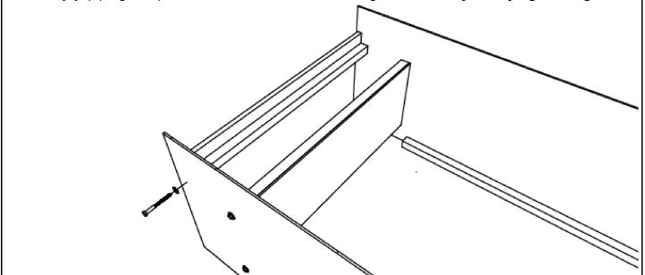
**Step 2 - A:** Loosely fasten side assemblies [A] to rear shelf support [G] using lag bolts [E] and flat washers [F], (1) lag bolt per side with a washer on each lag bolt. **Do not yet fully tighten lag bolts.**
