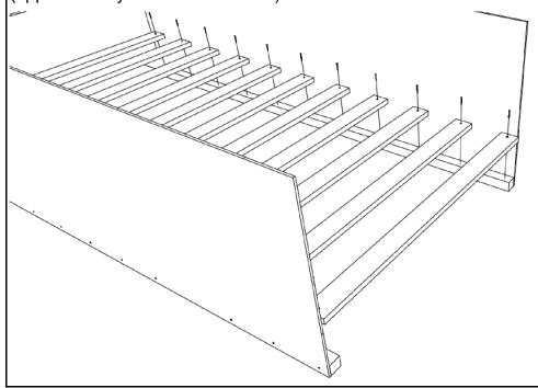
**Step 3 - B:** Fasten auxiliary side assemblies [A3] to side assemblies [A] and attached parts using screws [M]. Side assemblies pictured are for reference only; individual assembly types will vary with bed model. For exact fit and style, refer to picture on cover of manual.
