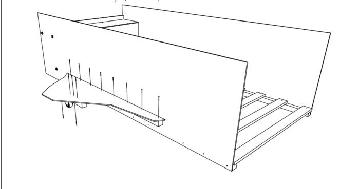
**Step 3 - J:** Fasten assemblies [A4] to shelf [H] using 3" long lag screws [M] and washers [F]. Use (1) washer [L] on each screw. Insert the lag screws through the side with the larger holes, and screw through the assembly towards the side with the smaller holes. Assemblies pictured are for reference only; individual assembly types will vary with bed model. For exact fit and style, refer to picture on cover of manual.
