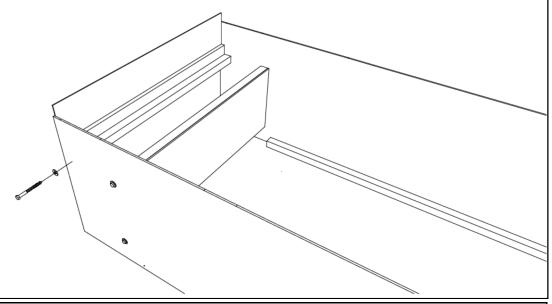
Step 2 - B: Fasten shelf [H] to headboard [D] and shelf rear support [G] with screws [l].
