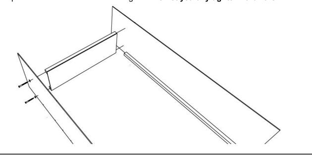
**Step 3:** Fasten mattress support bars [B] to support rail of side assemblies [A] using screws [C]. Use (1) screw at each end of support bar. Support bar end shall be perpendicular with side of bed. There may be a slight gap between end of support bar and side of bed. Start at rear of bed and work towards front. Leave approximately 4.5" gaps between each support bar (approximately 7" center-to-center).
