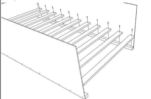
**Step 3 - C:** Fasten auxiliary side assemblies [A2] to side assemblies [A] using bolts [J] and nuts [K]. Use (1) washer [L] on each nut. Bolts shall face outward so that the smooth head is in. Side assemblies pictured are for reference only; individual assembly types will vary with bed model. For exact fit and style, refer to picture on cover of manual.
