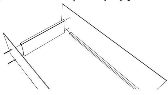
**Step 3:** Fasten mattress support bars [B] to support rail of side assemblies [A] using screws [C]. Use (1) screw at each end of support bar. Make sure support bar end is tight and perpendicular with side of bed. Start at rear of bed and work towards front. Leave 4.5" gaps between each support bar (approximately 7" center-to-center).
