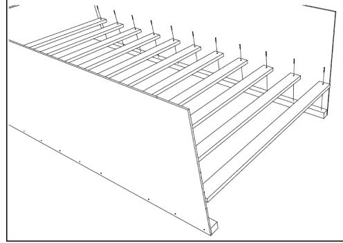
**Step 3 - C:** Fasten auxiliary side assemblies [A2] to side assemblies [A] using bolts [J] and nuts [K]. Use (1) washer [L] on each nut. Bolts shall face outward so that the smooth head is in. Side assemblies pictured are for reference only; individual assembly types will vary with bed model. For exact fit and style, refer to picture on cover of manual.
