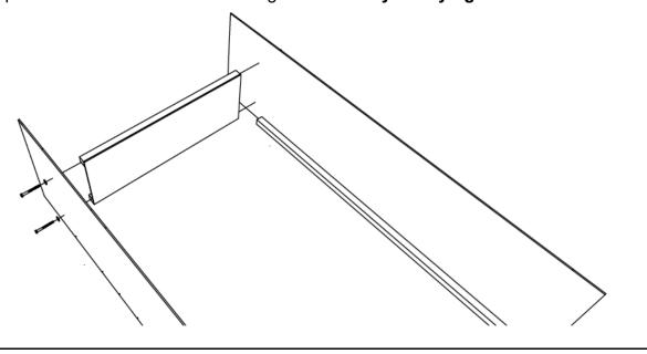
**Step 3:** Fasten mattress support bars [B] to support rail of side assemblies [A] using screws [C]. Use (1) screw at each end of support bar. Support bar end shall be perpendicular with side of bed. There may be a slight gap between end of support bar and side of bed. Start at rear of bed and work towards front. Leave approximately 4.5" gaps between each support bar (approximately 7" center-to-center).
