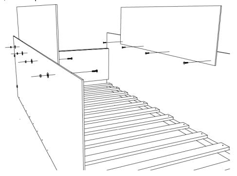
Fasten crossbars [A3-1] to auxiliary side assemblies [A3] using lag bolt [E]. Use (1) washer [F] on each lag bolt. Parts pictured are for reference only; individual assembly types will vary with bed model. For exact fit and style, refer to picture on cover of manual.
