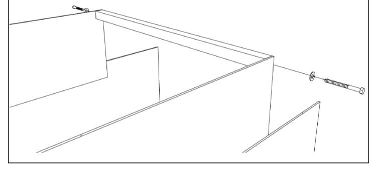
**Step 3 - Y:** Fasten auxiliary side assemblies [A2] to side assemblies [A] using bolts [J] and nuts [K]. Use (1) washer [L] on each nut. Bolts shall face outward so that the smooth head is in. Side assemblies pictured are for reference only; individual assembly types will vary with bed model. For exact fit and style, refer to picture on cover of manual.
