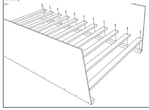
**Step 3 - T:** Fasten auxiliary side assemblies [A3] to side assemblies [A] using bolts [J] and nuts [K]. Use (1) washer [L] on each nut. Bolts shall face outward so that the smooth head is in. Side assemblies pictured are for reference only; individual assembly types will vary with bed model. For exact fit and style, refer to picture on cover of manual.
