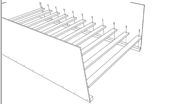
**Step 3 - E:** Fasten auxiliary side assemblies [A1] and [A2] to side assemblies [A] using bolts [J] and nuts [K]. Use (1) washer [L] on each nut. Bolts shall face outward so that the smooth head is in. Side assemblies pictured are for reference only; individual assembly types will vary with bed model. For exact fit and style, refer to picture on cover of manual.
