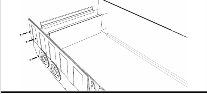
**Step 3:** Fasten shelf [E] to shelf front section [C] and shelf rear section [D] using (18) screws [H].
