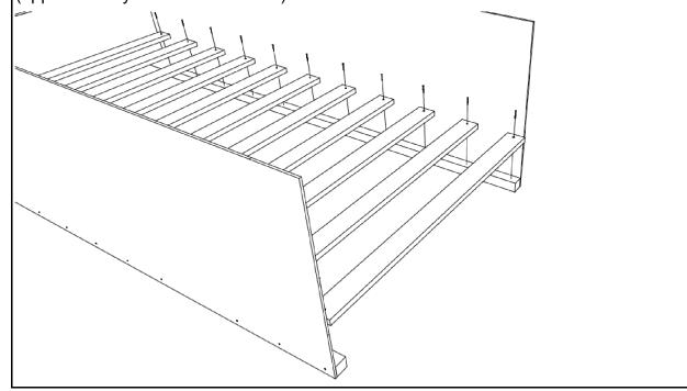
**Step 3 - A:** Fasten auxiliary side assemblies [A2] to side assemblies [A] using bolts [J] and nuts [K]. Use (1) washer [L] on each nut. Bolts shall face outward so that the smooth head is in. Side assemblies pictured are for reference only; individual assembly types will vary with bed model. For exact fit and style, refer to picture on cover of manual.
