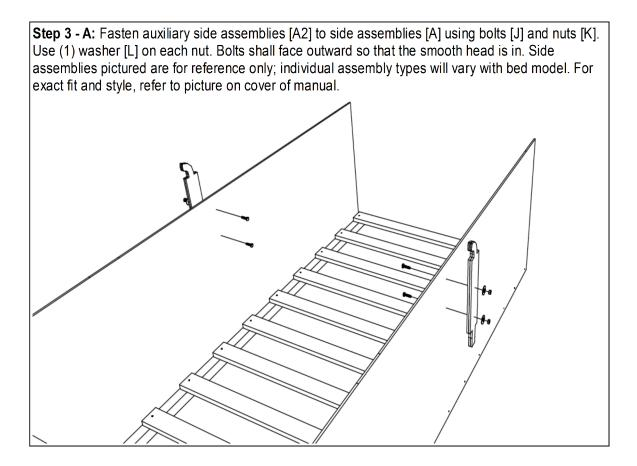
**Step 3 - E:** Fasten auxiliary side assemblies [A2] to side assemblies [A] using bolts [J] and nuts [K]. Use (1) washer [L] on each nut. Bolts shall face outward so that the smooth head is in. Side assemblies pictured are for reference only; individual assembly types will vary with bed model. For exact fit and style, refer to picture on cover of manual.
