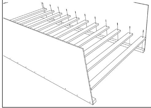
**Step 3 - A:** Fasten auxiliary side assemblies [A2] to side assemblies [A] using bolts [J] and nuts [K]. Use (1) washer [L] on each nut. Bolts shall face outward so that the smooth head is in. Side assemblies pictured are for reference only; individual assembly types will vary with bed model. For exact fit and style, refer to picture on cover of manual.
