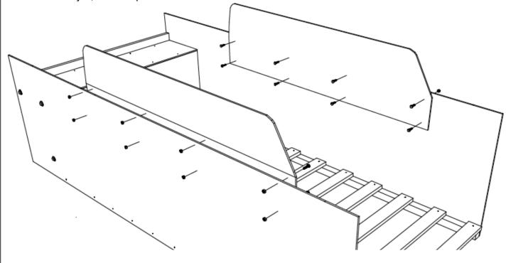
**Step 3 - L:** Fasten cab crossbars [A3] to auxiliary side assemblies [A2] using lag bolt [E]. Use (1) washer [F] on each lag bolt. Parts pictured are for reference only; individual assembly types will vary with bed model. For exact fit and style, refer to picture on cover of manual.
