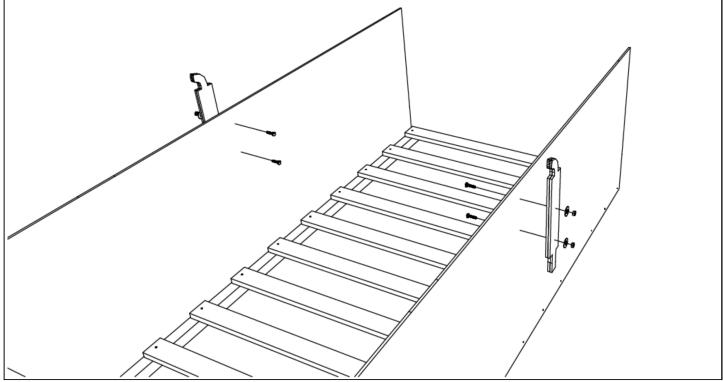
**Step 3 - E:** Fasten auxiliary side assemblies [A2] to side assemblies [A] using bolts [J] and nuts [K]. Use (1) washer [L] on each nut. Bolts shall face outward so that the smooth head is in. Side assemblies pictured are for reference only; individual assembly types will vary with bed model. For exact fit and style, refer to picture on cover of manual.
