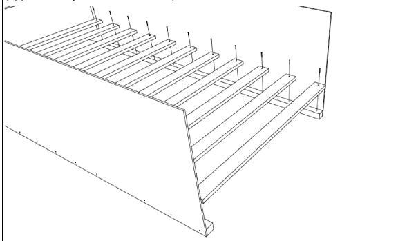
**Step 3 - A:** Fasten auxiliary side assemblies [A2] to side assemblies [A] using bolts [J] and nuts [K]. Use (1) washer [L] on each nut. Bolts shall face outward so that the smooth head is in. Side assemblies pictured are for reference only; individual assembly types will vary with bed model. For exact fit and style, refer to picture on cover of manual.
