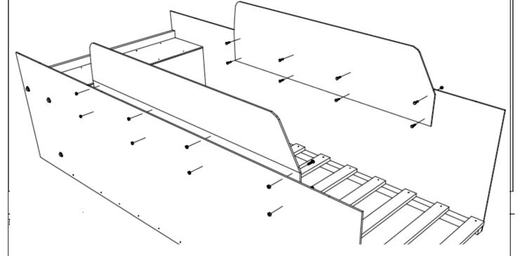
**Step 3 - L:** Fasten cab crossbars [A3-1] to auxiliary side assemblies [A3] using lag bolt [E]. Use (1) washer [F] on each lag bolt. Parts pictured are for reference only; individual assembly types will vary with bed model. For exact fit and style, refer to picture on cover of manual.
