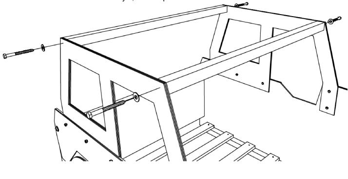
**Step 3 - M:** Fasten footboard shelf ends to upper shelf using lag bolts [E]. Use (1) washer [F] on each lag bolt. Fasten front of lower shelf to shelf ends using lag bolt [E] and one washer [F]. Fasten rear of lower shelf to shelf ends (through runner) using longer lag bolt [A4-2] and one washer [F].
