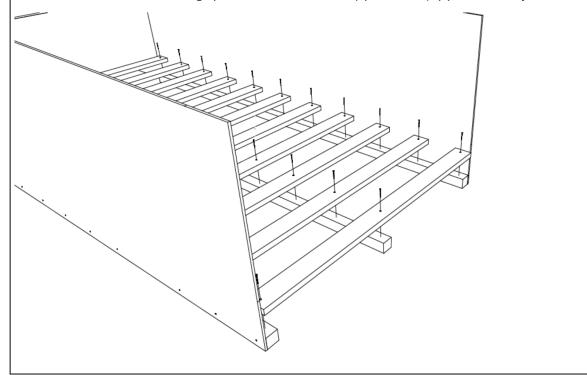
Step 3 - H: Fasten auxiliary assembly [A2] to headboard assembly [A] using bolts [J] and nuts [K]. Use (1) washer [L] on each nut. Bolts shall face outward so that the smooth head is in. Side assemblies pictured are for reference only; individual assembly types will vary with bed model. For exact fit and style, refer to picture on cover of manual.
