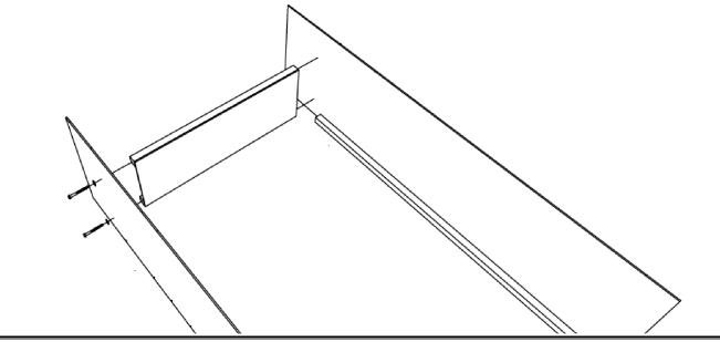
**Step 2 - A:** Loosely fasten side assemblies [A] to rear shelf support [G] using lag bolts [E] and flat washers [F], (1) lag bolt per side with a washer on each lag bolt. **Do not yet fully tighten lag bolts.**
