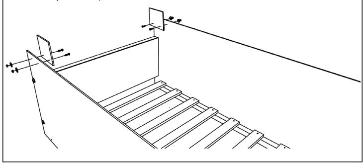
Step 4: Tighten all hardware. Make sure all assembled parts are tight and secure.
