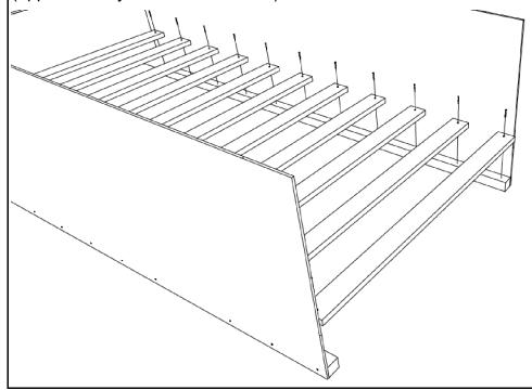
**Step 3 - I:** Fasten auxiliary side assemblies [A2] to side assemblies [A] using bolts [J] and nuts [K]. Use (1) washer [L] on each nut. Bolts shall face outward so that the smooth head is in. Side assemblies pictured are for reference only; individual assembly types will vary with bed model. For exact fit and style, refer to picture on cover of manual.
