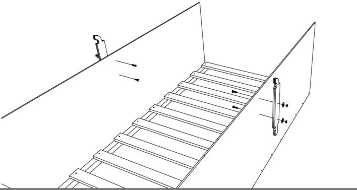
**Step 3 - B:** Fasten auxiliary side assemblies [A3] to side assemblies [A] and attached parts using screws [M]. Side assemblies pictured are for reference only; individual assembly types will vary with bed model. For exact fit and style, refer to picture on cover of manual.
