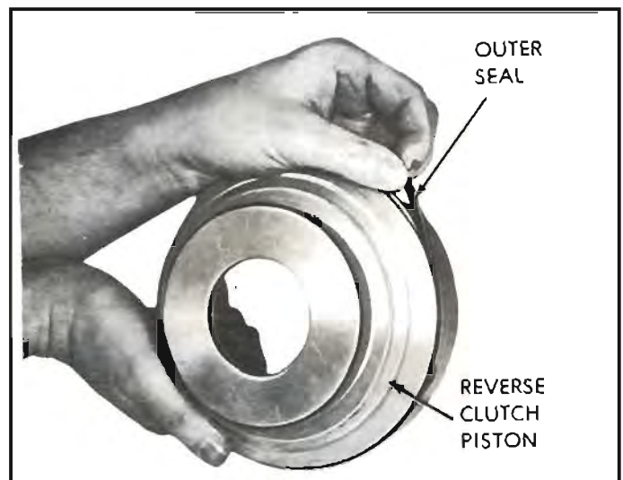
Figure 78 Outer Seal Installation
