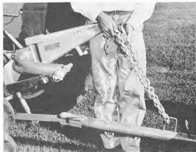
Fig. 30 - Installing Coupler Chain to Implement
