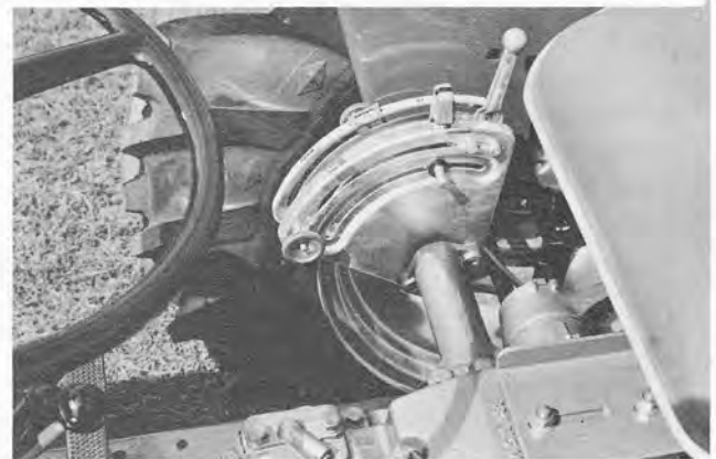
Fig. 8 - Hydraulic Quadrant - Without Pressure Control
