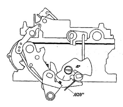
Crack the throttle valves and manually open and close the choke valve. The tang on the secondary throttle lever should freely engage in the notch of the lock out dog. To adjust, bend the tang on the secondary throttle lever.
