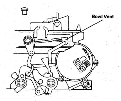
The AFB series emission calibrated carburetors use a combination of a mechanically operated internal and external vents. The non-emission calibrated and marine carburetors use an internal vent only.
