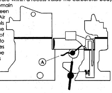
When the accelerator is fully depressed, only the primary high speed circuit will function until there is sufficient air velocity to open the auxiliary valves. When this occurs, fuel will then come from the secondary high-speed circuit.
