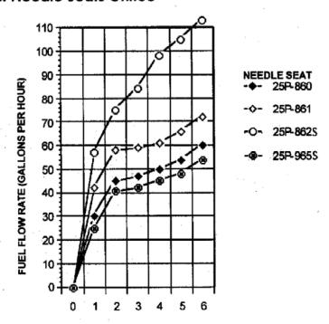
FUEL PRESSURE (PSI) HIGH RPM CONDITIONS
