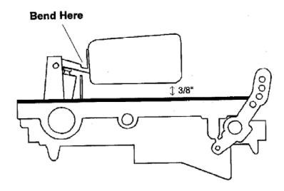
With the bowl cover inverted, bowl cover gasket in place, and weight of float seating on the needle, there should be 3/8" between the top of each float and the bowl cover gasket (at the outer end on the seam). The sides of the floats should be parallel to the outer edge of the bowl cover. To adjust, bend the float lever near the pivot pin.
