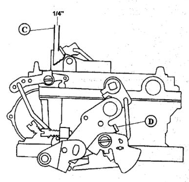
With the throttle valves open, close the choke valve as far as possible without forcing. The dimension (C) between the top edge of the choke valve and the inner wall of air horn should be 1/4". To adjust, bend the tang (D) on the throttle lever.
