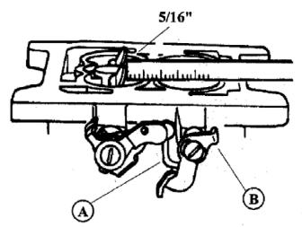
Secondary throftle valves should just start to open when there is 5/16" between the primary throftle valve and the bore of the carburetor as shown. To adjust bend rod (A). With the primary throftle valves wide open, adjust the stop tang (B) until the secondary valves are 27/32" from the edge of the bore before full vertical position.
