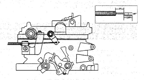
Mount knob assembly (CARTER #9600C) in a convenient location under the dash. Next install the cable through the firewall of the engine compartment. Trim the cable to the approximate length plus 6 inches.
