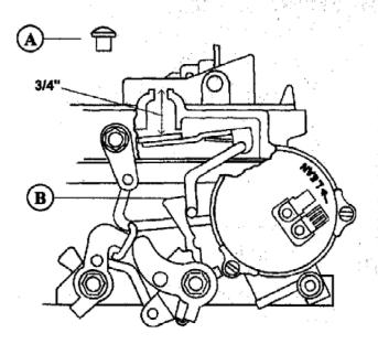
Remove the plug (A) from the hole in the air horn and insert a narrow ruler. Allow the rule to rest lightly on the top of the valve. With the throttle valves closed and choke open, the dimension from the top of the valve to the top of the hole should able 3/4". To adjust, bend the operating lever (B).
