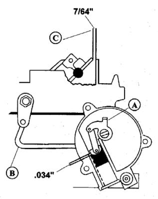
Open the choke valve and insert a .034" wire (paper clip) (bend 90 degrees 1/8" from the end) between top of slot in the choke piston cylinder and the bottom of the slot in the piston. Hold the wire in position and close choke valve by pressing on the piston (A) until resistance is felt. The dimension (C) should be 7/64" between the top edge of the choke valve and the wall of the air horn. To adjust bend rod (B). Reassemble the thermostatic choke coil to the housing.
