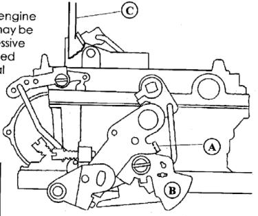
If oil is used, it will attract dirt, become gummy and interfere with correct linkage operation.
