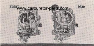
As a special option, the 409 cubic inch engine may be equipped with TWO AFB carburetars. The front model is 33615 and the rear model, containing a choke assembly, is designated 33625. Both have air horn throat diameters of 4½ inches. Chevrolet part numbers are 3815403 and 3815404.
