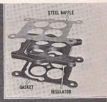
409 cubic inch engine uses only the gasket.
