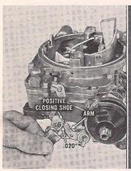
With the choke blocked wide open, close the primary throttle valves tightly. There should be a .020" clearance between the positive closing shoe of the secondary valves and the primary throttle shaft arm. If necessary, bend the positive closing shoe to obtain correct clearance.
