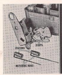
Check the steps on the fast idle cam for excessive wear and all movable linkage parts for an out-of-round condition or enlargement of the pivoting holes. Inspect vacuum-operated pistons and metering rods for damage.
