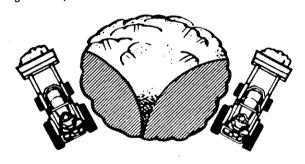
If the sides of the pile are too high, use the loader to pull down the sides and to reduce the possibility of stockpile slides.
