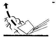
a level bucket throughout the lifting cycle resists bucket lift or breakaway.
