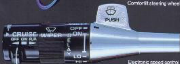
Electronic speed control and intermittent wiper shown on standard multi-function switch.
