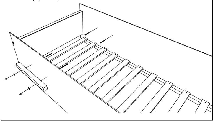
**Step 3 - G:** Fasten auxiliary side assemblies [A3] to auxiliary side assemblies [A2] using lag bolt [M]. Use (1) washer [L] on each lag bolt. Side assemblies pictured are for reference only; individual assembly types will vary with bed model. For exact fit and style, refer to picture on cover of manual.
