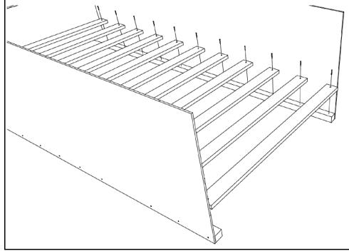
**Step 3 - F:** Fasten auxiliary side assemblies [A2] to side assemblies [A] using bolts [J] and nuts [K]. Use (1) washer [L] on each nut. Bolts shall face outward so that the smooth head is in. Side assemblies pictured are for reference only; individual assembly types will vary with bed model. For exact fit and style, refer to picture on cover of manual.
