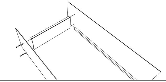
Step 2 - A: Loosely fasten side assemblies [A] to rear shelf support [G] using lag bolts [E] and flat washers [F], (1) lag bolt per side with a washer on each lag bolt. Do not yet fully tighten lag bolts.
