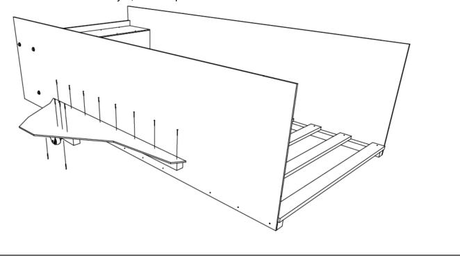
**Step 3 - V:** Fasten auxiliary rear assembly [A2] to back of headboard [D] using 3" long lag screws [N] and washers [F]. Use (1) washer on each screw. Insert the lag screws through the side with the larger holes, and screw through the assembly towards the side with the smaller holes. Assemblies pictured are for reference only; individual assembly types will vary with bed model. For exact fit and style, refer to picture on cover of manual.
