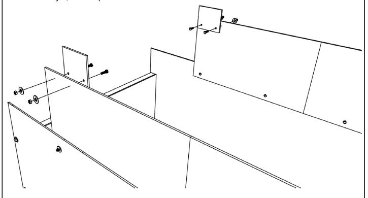
**Step 3 - Q:** Fasten crossbars [A5] between sides using lag screws [E]. Use (1) washer on each screw.
