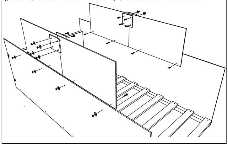
**Step 3 - O:** Fasten side assembles [A4] to side assembly [A3] using carriage bolts [J]. Use (1) washer [L] and one nut [K] on each bolt. Bolts shall face outward so that the smooth head is in. Side assemblies pictured are for reference only; individual assembly types will vary with bed model. For exact fit and style, refer to picture on cover of manual.
