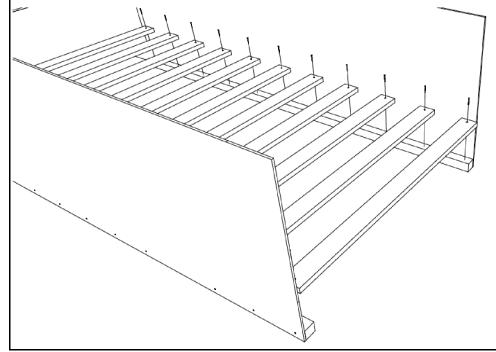
**Step 3 - O:** Fasten side assembles [A2] to side assembly [A] using connector plate [A3] on each side. Use carriage bolts [J]. Use (1) washer [L] and one nut [K] on each bolt. Bolts shall face outward so that the smooth head is in. Side assemblies pictured are for reference only; individual assembly types will vary with bed model. For exact fit and style, refer to picture on cover of manual.
