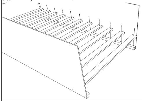
**Step 3 - D:** Fasten auxiliary side assemblies [A2] to side assemblies [A] using bolts [J] and nuts [K]. Use (1) washer [L] on each nut. Bolts shall face outward so that the smooth head is in. Side assemblies pictured are for reference only; individual assembly types will vary with bed model. For exact fit and style, refer to picture on cover of manual.
