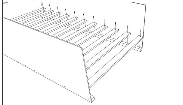
**Step 3 - D:** Fasten auxiliary side assemblies [A2] to side assemblies [A] using bolts [J] and nuts [K]. Use (1) washer [L] on each nut. Bolts shall face outward so that the smooth head is in. Side assemblies pictured are for reference only; individual assembly types will vary with bed model. For exact fit and style, refer to picture on cover of manual.
