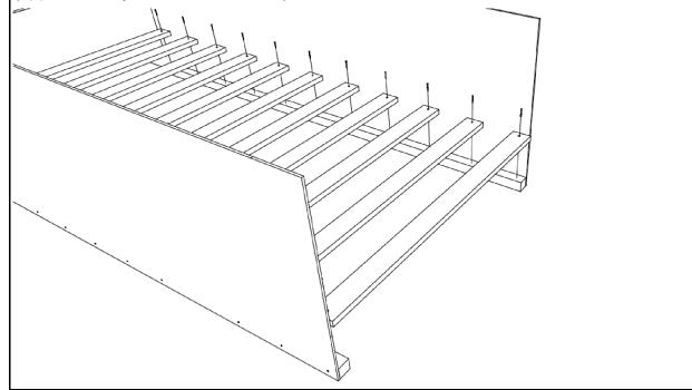
**Step 3 - C:** Fasten auxiliary side assemblies [A2] to side assemblies [A] using bolts [J] and nuts [K]. Use (1) washer [L] on each nut. Bolts shall face outward so that the smooth head is in. Side assemblies pictured are for reference only; individual assembly types will vary with bed model. For exact fit and style, refer to picture on cover of manual.
