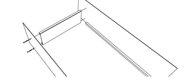
**Step 3:** Fasten mattress support bars [B] to support rail of side assemblies [A] using screws [C]. Use (1) screw at each end of support bar. Make sure support bar end is tight and perpendicular with side of bed. Start at rear of bed and work towards front. Leave 4.5" gaps between each support bar (approximately 7" center-to-center).
