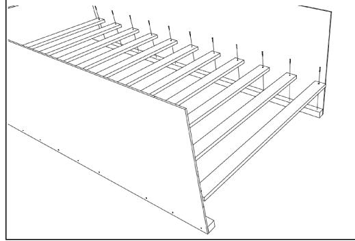
**Step 3 - A:** Fasten auxiliary side assemblies [A2] to side assemblies [A] using bolts [J] and nuts [K]. Use (1) washer [L] on each nut. Bolts shall face outward so that the smooth head is in. Side assemblies pictured are for reference only; individual assembly types will vary with bed model. For exact fit and style, refer to picture on cover of manual.
