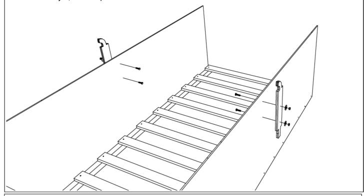
**Step 3 - E:** Fasten auxiliary side assemblies [A3] to side assemblies [A] using bolts [J] and nuts [K]. Use (1) washer [L] on each nut. Bolts shall face outward so that the smooth head is in. Side assemblies pictured are for reference only; individual assembly types will vary with bed model. For exact fit and style, refer to picture on cover of manual.
