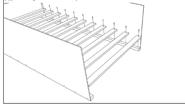
Step 3 - H: Fasten auxiliary assembly [A2] to headboard assembly [A] using bolts [J] and nuts [K]. Use (1) washer [L] on each nut. Bolts shall face outward so that the smooth head is in. Side assemblies pictured are for reference only; individual assembly types will vary with bed model. For exact fit and style, refer to picture on cover of manual.
