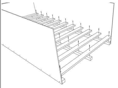
**Step 3 - A:** Fasten auxiliary side assemblies [A2] to side assemblies [A] using bolts [J] and nuts [K]. Use (1) washer [L] on each nut. Bolts shall face outward so that the smooth head is in. Side assemblies pictured are for reference only; individual assembly types will vary with bed model. For exact fit and style, refer to picture on cover of manual.
