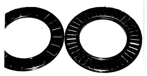
Early TH 400s used a 20-needle bearing assembly on both sides of the planetary sun gear and between the rear ring gear and output shaft. These should be upgraded to the later 40-needle bearing sets for obvious reasons.
