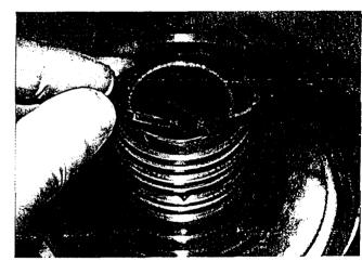
Replace all Teflon sealing rings with the cast-iron upgrades. Their temperature and pressure capacities are bulletproof.
