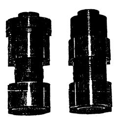
The valve shown on the right here is TransGo's upgrade to keep the transmission from shifting to Second even when held in manual Low. With the land on the valve gone and a plug inserted into the valve body casting, any gear can be selected at any time for manual control.
