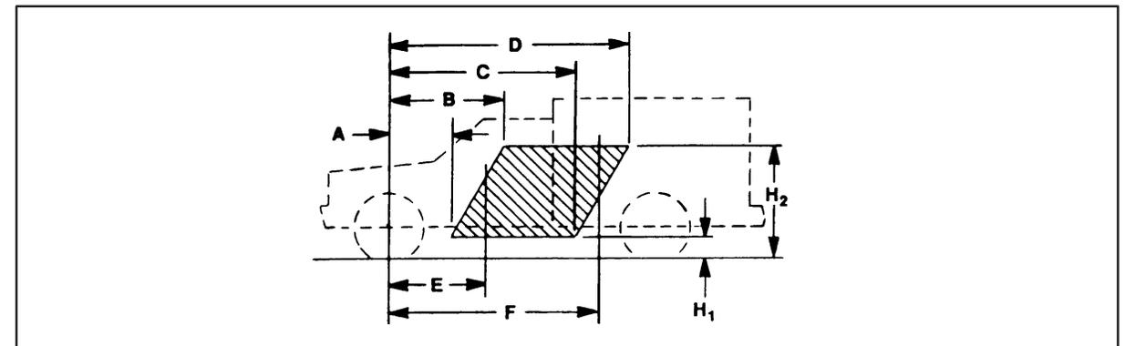
**C.G. of vehicle in FMVSS unladen condition (Curb + 400 lbs.) must be inside shaded area – that is, it must be within the trapezoid formed by the coordinates A, B C, D, H<sub>1</sub> & H<sub>2</sub>, plus it must be to the rear of vertical line E and forward of vertical line F.**
