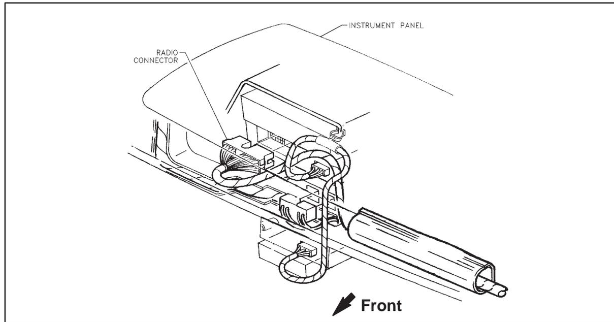
The radio may have to be removed from the instrument panel to gain access to the 20 pin connector.
