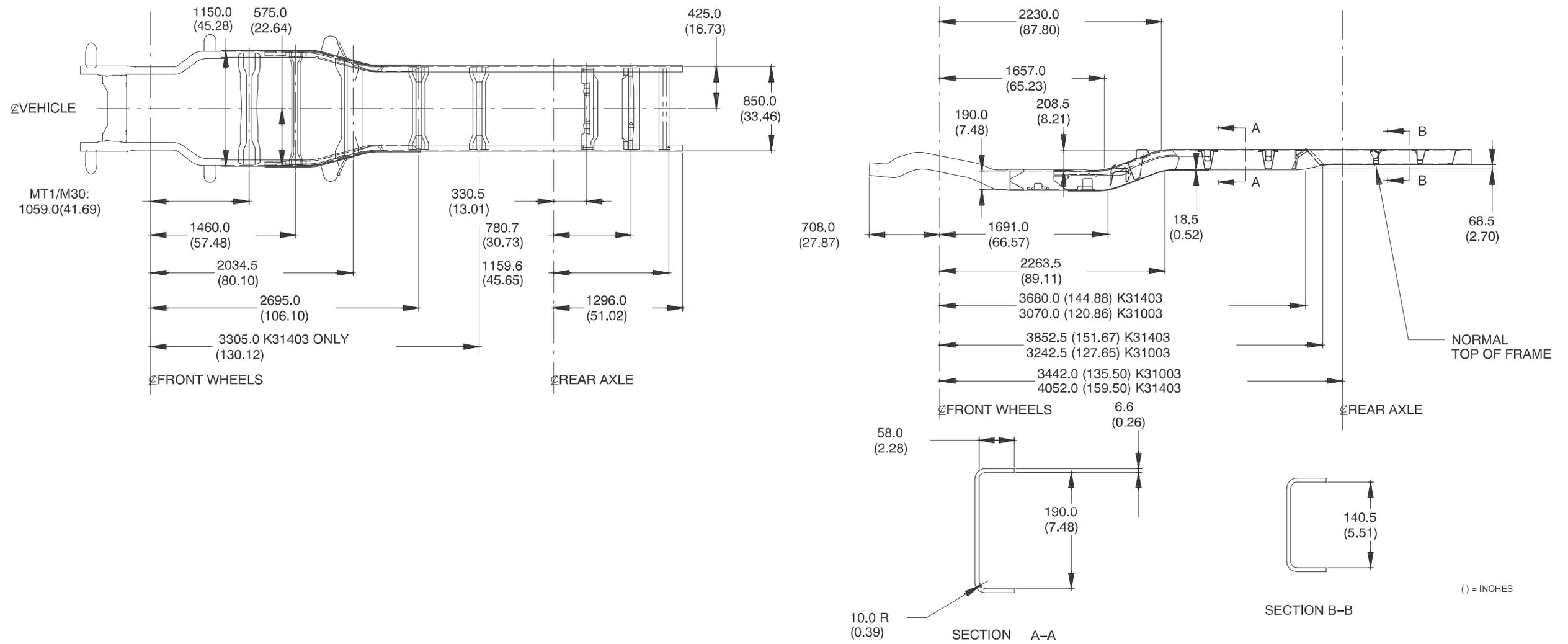
K (310/314)03 Chassis Cab, 12,000 lb. GVWR, Frame Reinforcement
