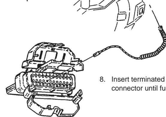
8. Insert terminated lead into cavity "2" of connector until fully seated.
