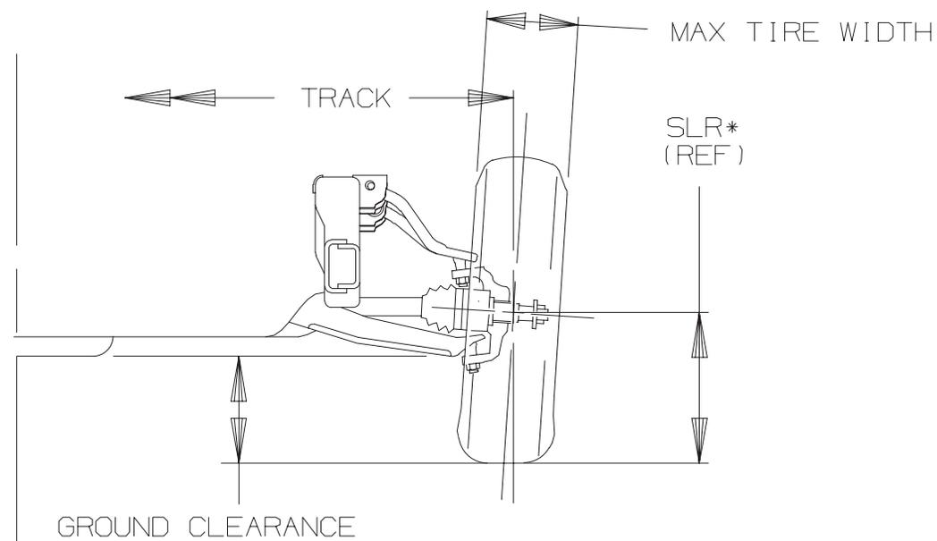
\*MINIMUM GROUND CLEARANCE TO BE CALCULATED BY USING GROSS AXLE WEIGHT AND RECOMMENDED TIRE PRESSURE
