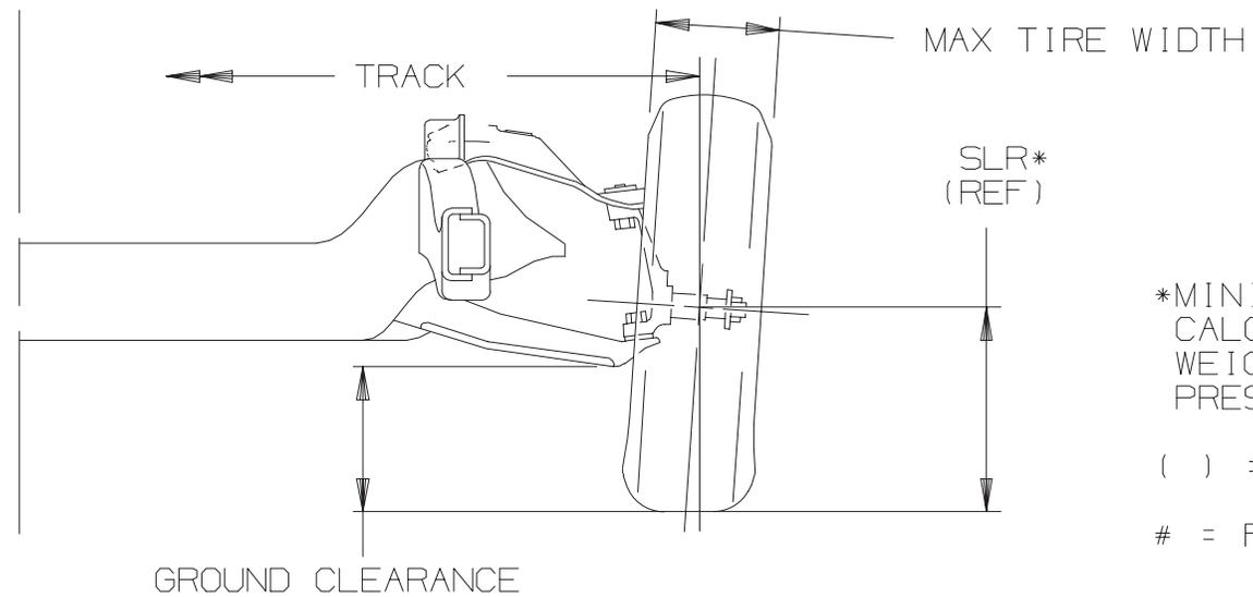
\*MINIMUM GROUND CLEARANCE TO BE CALCULATED BY USING GROSS AXLE WEIGHT AND RECOMMENDED TIRE PRESSURE
