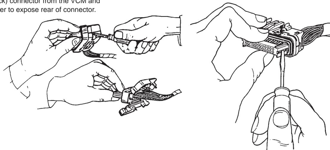
5. Remove Terminal Position Assurance (TPA) clip from front of connector.
