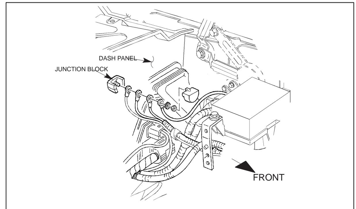
Also, for cab/chassis with the "YF2" option, heavy gauge ground straps have been provided between the engine, chassis and body sheet metal near the right rear of the engine for the purpose of providing a robust ground return path from the body or chassis to the battery. The body builder must ensure that the ground returns from their loads provide an adequate ground path into these straps such that voltage drops are minimized.
